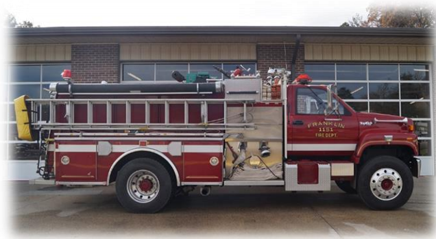
1151 1993 GMC TopKick EEI Pumper 750 Gallon Tank and 1250 GPM Hale Pump. It is used on structure fires.
