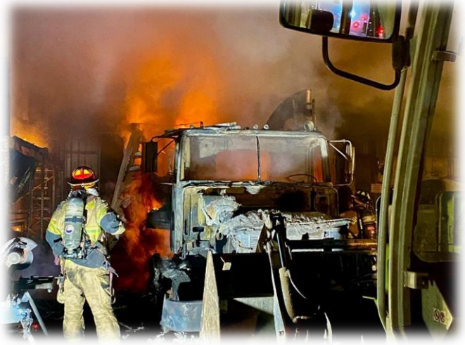
Diesel fuel and hydraulic fluids exacerbated the fire
